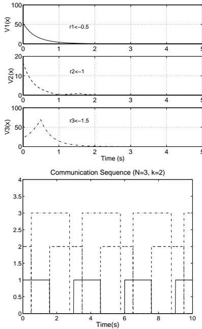
**Figure 3:** Systems 2 and 3 have faster guaranteed convergence rates resulting from the allocation of more network time to them.
