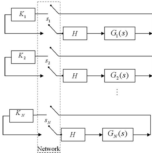
**Figure 1:** A collection of networked control systems  $G_i(s) = I(sI - A_i)^{-1}B_i$  driven by feedback controllers  $K_i$  via a network.  $H$  denotes a zero-order-hold stage. Only  $k$  of  $N$  switches  $s_i$  can be closed at any one time.
